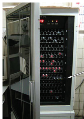
Figure-2: Photograph showing the automated incubator used for MB/Bact culture bottles with indicators showing culture bottles which have flashed positive (arrow)
