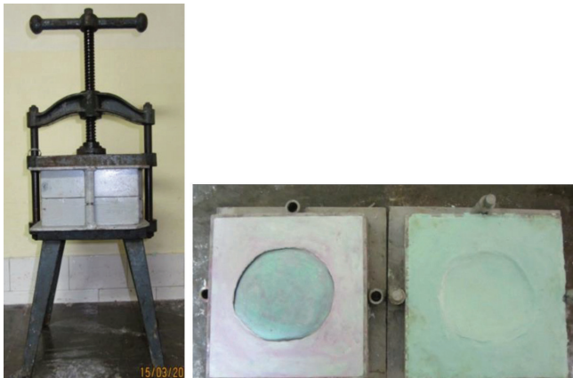
Figure-2: (a) Custom made compression clamp; (b) Custom made flask
